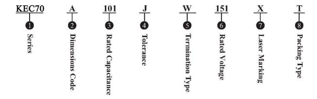
① Series: Kete 70 Series High Q High Power Capacitor, Temperature Coefficient:  $0 \pm 30$ ppm/°C.
